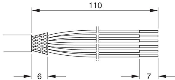
1. Strip the cable ends by approx. 110 mm and shorten the cable shield to 6 mm.
