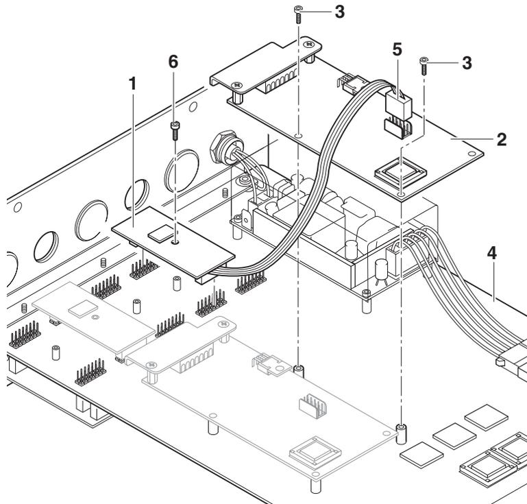
1. Remove the blind plug from the desired interface connection (X6, X7 or X8).
