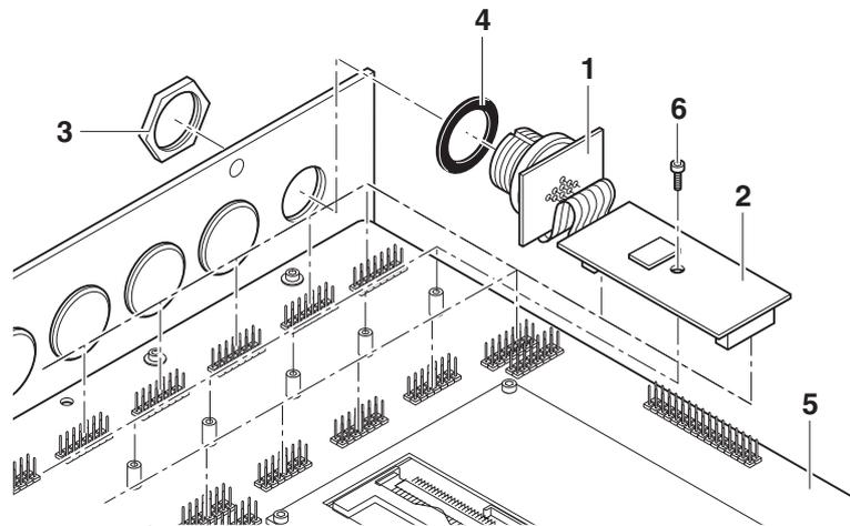
1. Remove the blind plug from the desired interface connection.
