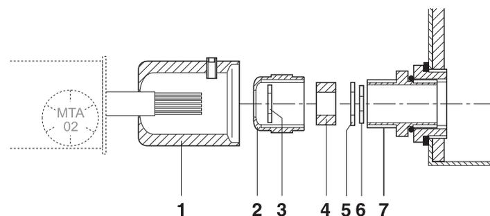
1. Slide the sealing sleeve (1), union nut (2), washer (3), moulded seal (4) and contact washer with large bore size (5) over the cable sheathing. If any braided screen cores loosen in the process, these may not contact any conductive system parts!
