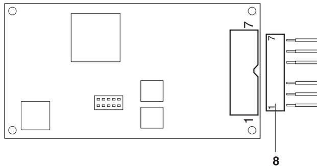
2. Pull the connector (8) from the analog PCB and terminate the cores of the weighing platform cable at the connector as follows:
